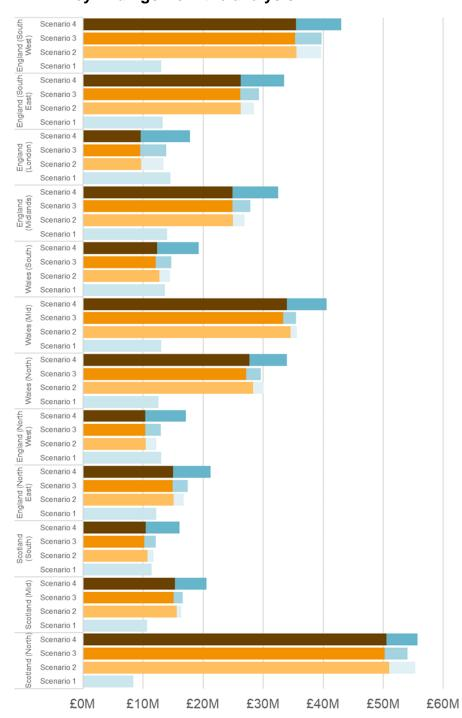
Network infrastructure costs per household are, on average likely to be much higher for hydrogen than for electrification. Network infrastructure reinforcement costs vary significantly by location for both electricity and gas network reinforcement. The variation between different regions is more pronounced for gas networks cost than electricity network costs.
